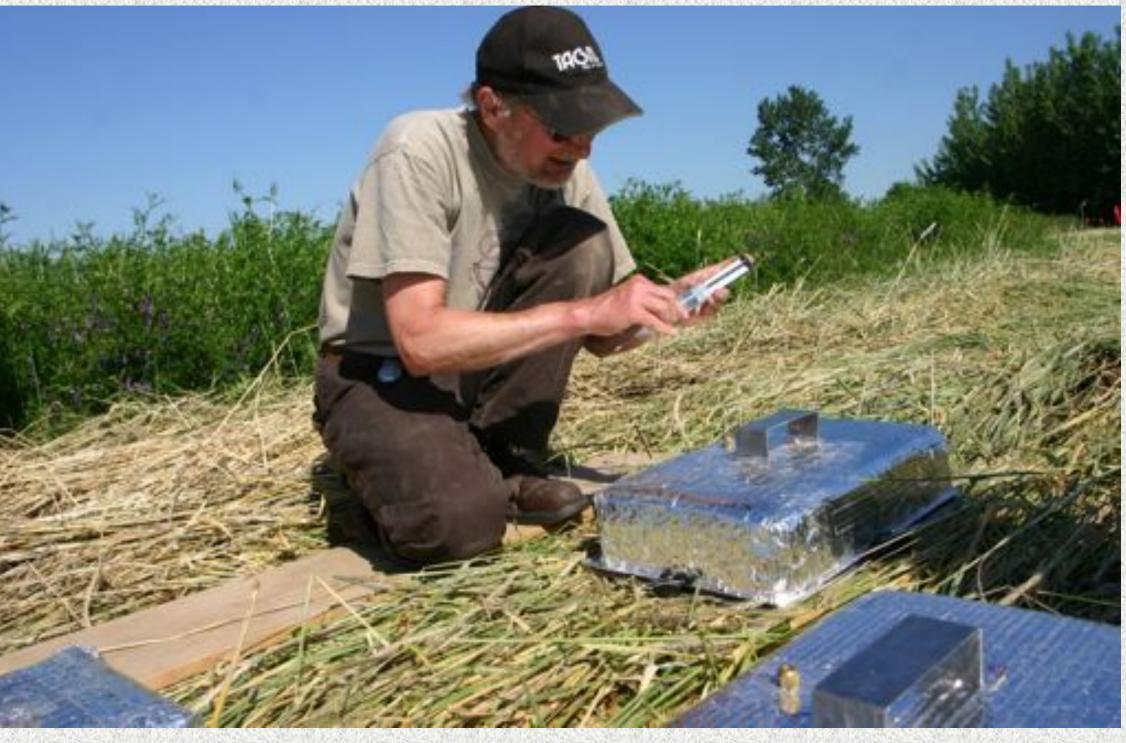
Figure 5. Sampling gas for nitrous oxide and carbon dioxide flux measurements from chambers in reduced tillage organic plots.
